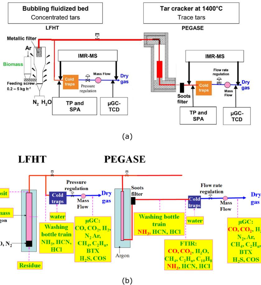
Figure 95. Schematic view of the pilot scale facilities LFHT linked to PEGASE, including gas analysis points: (a) analysis of tars and permanent gas (IMR-MS, micro-GC, Tar Protocol (TP) and SPA); (b) measurement of inorganics (FTIR, micro-GC, wet chemical analysis) [167].
