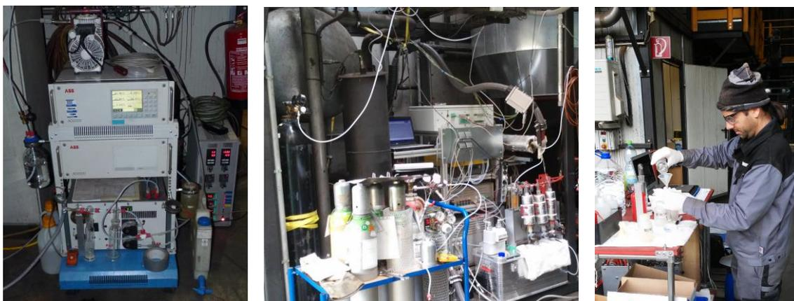
Figure 97. Multi-component gas analyser for permanent gases (left) applied at BE2020+: FTIR including gas dilution unit and tar sampling (middle); sample processing for wet chemical analysis (right) [205].
