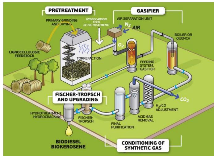
Figure 71. Schematic view of the BioTfuel thermochemical conversion route [166].
