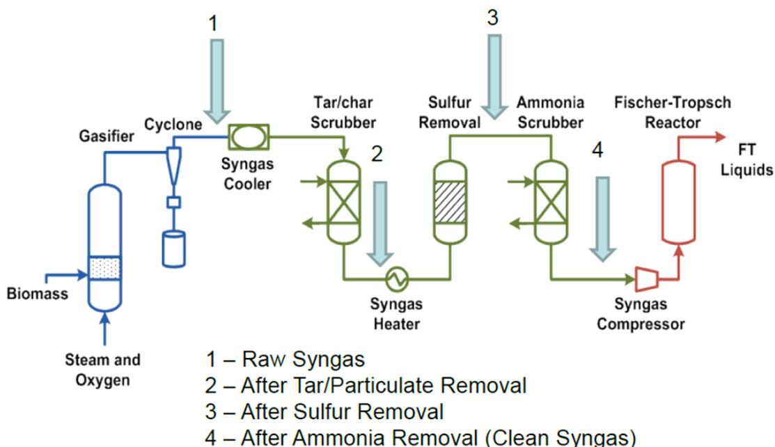
Figure 84. Schematic of the biomass gasification to biofuel located at Iowa State University [76][172].
