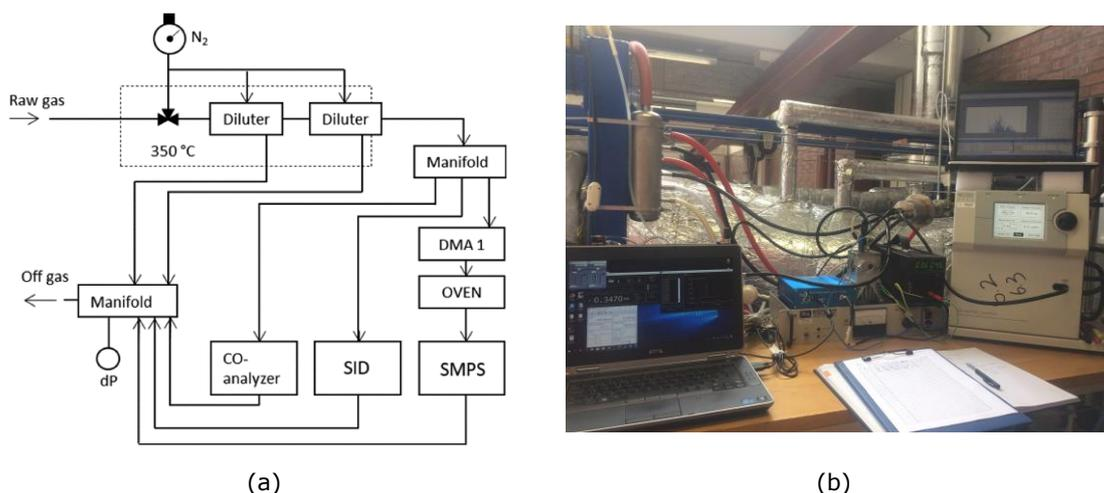
Figure 33. (a) Schematic layout of the setup for the online measurement of alkali metals in product gas applied by Gothenburg University at the GoBiGas plant [126]; (b) implementation of the SID, picture courtesy of Gothenburg University.
