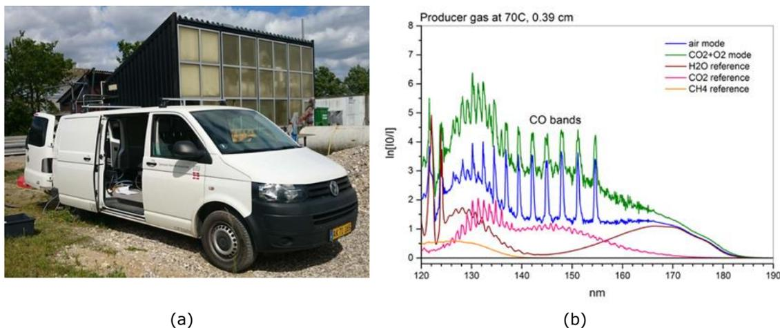
Figure 66. Optical measurements applied at the Viking gasifier by DTU [122].
