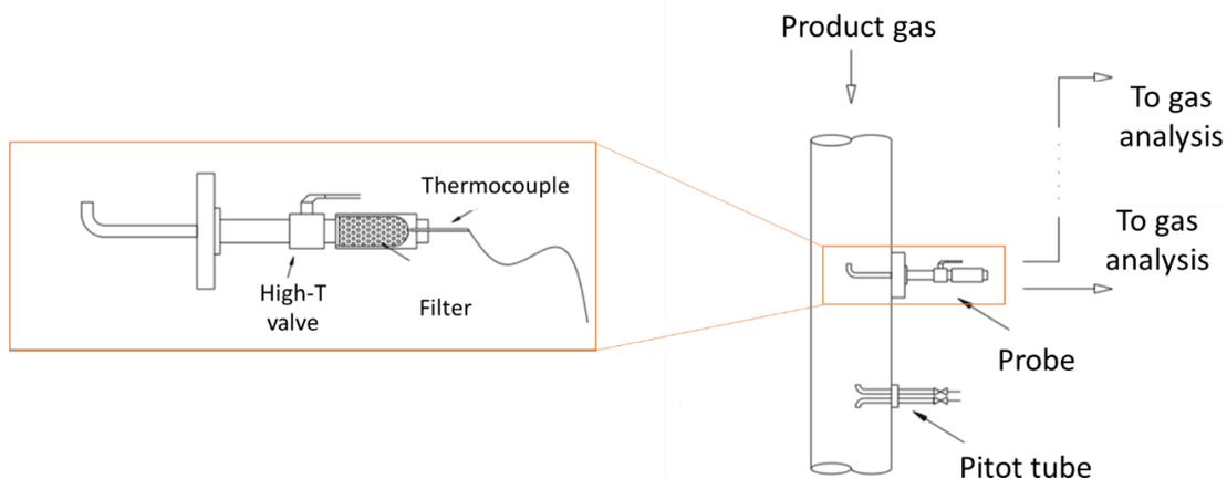
Figure 89. Schematic layout of gas sampling at BFB pilot plant at University of Seville [85].
