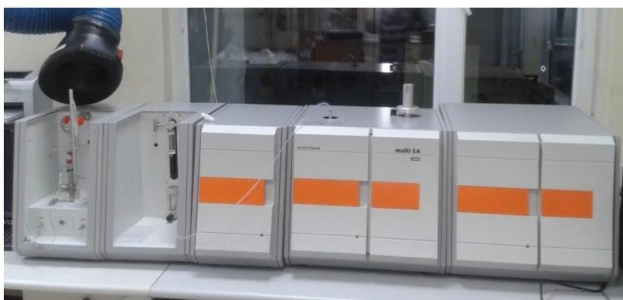
Figure 23. UV fluorescence total sulphur analyser. Picture courtesy of Tübitak Mam [80].
