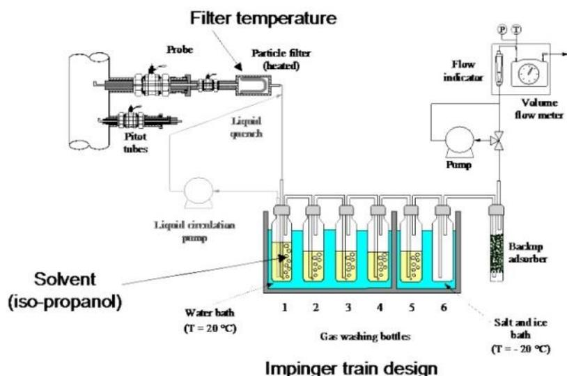
Figure 15. Schematic of tar sampling train according to the tar guideline [37][42].
