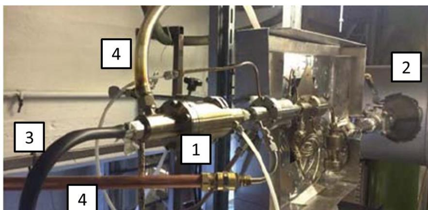
Figure 32. Sampling probe for cooling and dilution of product gas applied by Gothenburg University for online measurement of alkali compounds and heavy tars [125]: 1: Ejector diluters; 2: Raw gas line; 3: Diluted sample gas; 4: Off-gases.
