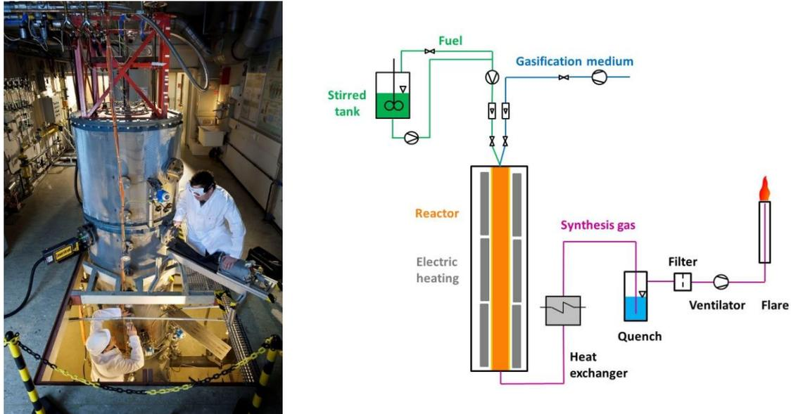
Figure 79. Picture and process flow scheme of the REGA bench-scale gasifier [159].
