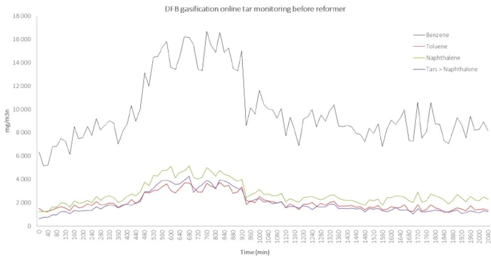
Figure 19. Results of rapid tar measurement applied by VTT [19].
