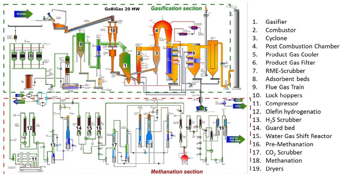
Figure 53. Schematic of GoBiGas plant [60].
