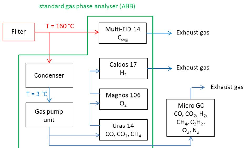
Figure 80. Setup of gas sampling system used at the REGA setup [159].
