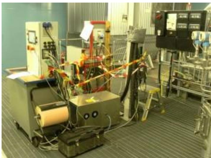
Figure 104. CON-TAR online tar measurement unit at the GoBiGas plant. Picture courtesy of Goteborg Energi [60].
