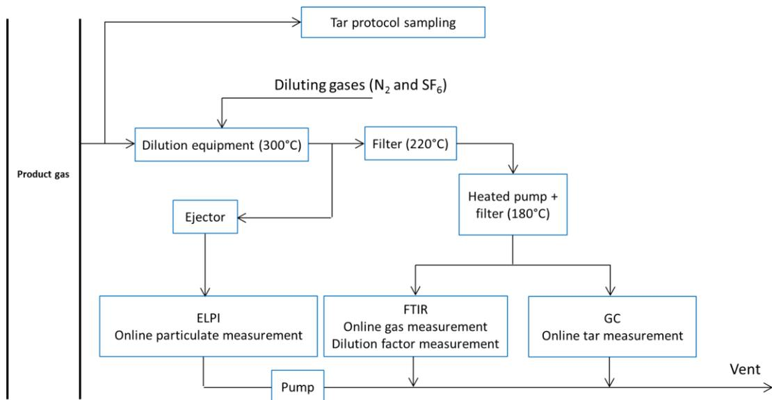
Figure 8. Schematic layout of gas conditioning and analysis equipment for online measurement of particles, gas and tar at VTT [19].
