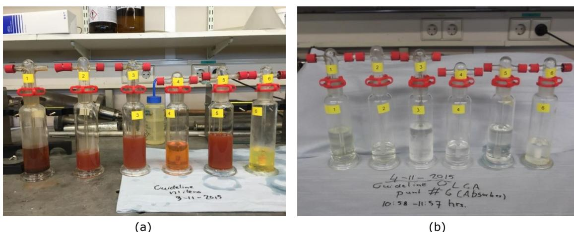
Figure 16. Impingers after tar guideline sampling: (a) raw MILENA product gas; (b) Gas after OLGA tar removal. Picture courtesy of ECN part of TNO.
