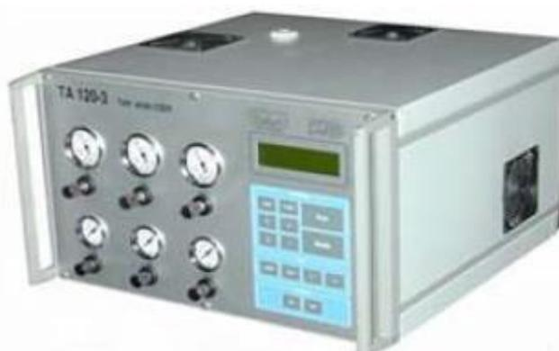
Figure 103. Commercial online tar analyser developed by University of Stuttgart [57][210][211].
