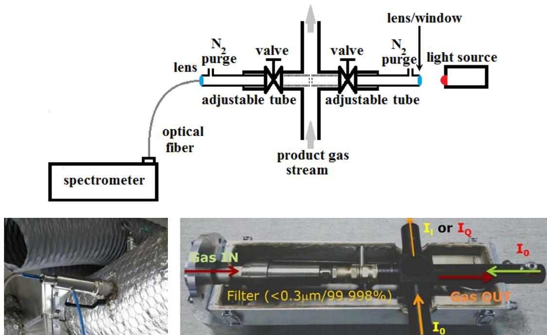
Figure 110. In-situ UV measurement of tars (no gas extraction) by DTU [11][65][122][219].
