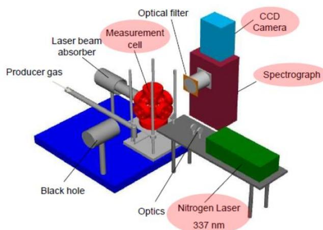
Figure 107. Laser Induced Fluorescence Spectroscopy [58].
