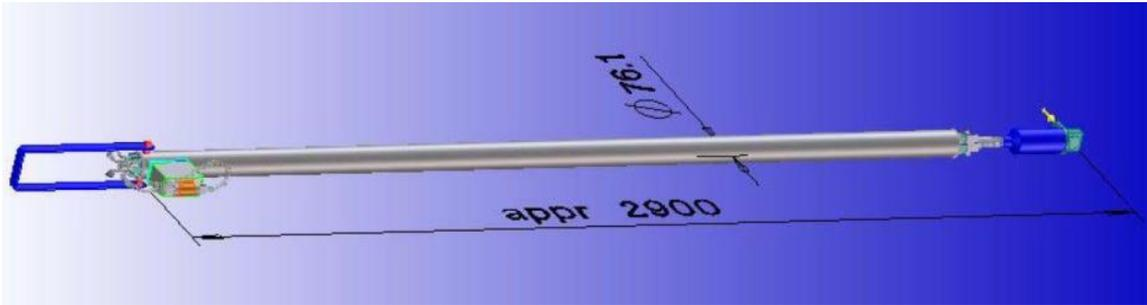
Figure 41. Schematic of the dust sampling probe configured for in-duct cascade impactor measurement used at ECN part of TNO [142]. Dimensions in mm.
