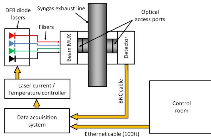
Figure 114. Schematic diagram of TDLAS unit developed by University of Stanford and University of Utah and implementation in gasification line [14].
