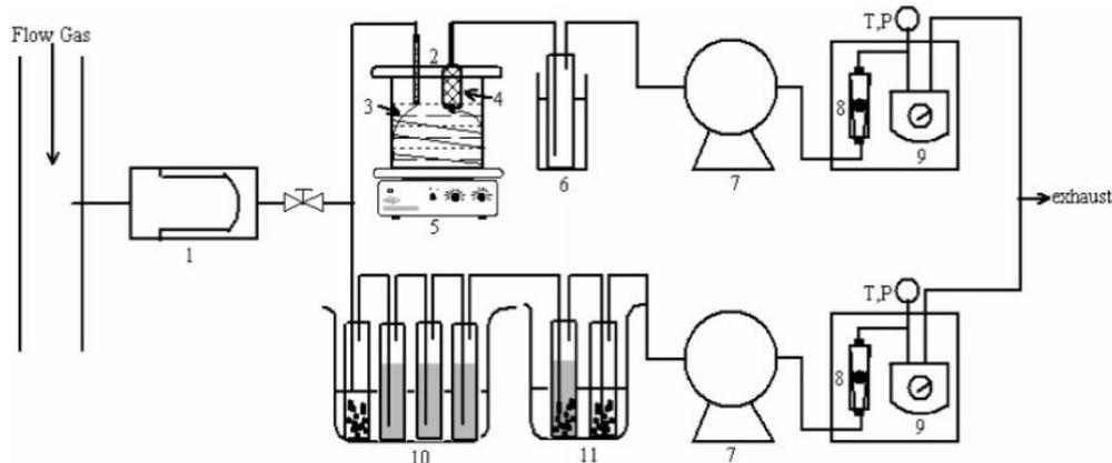
Figure 17. Schematic of the tar sampling and collection system used at Iowa State University. The upper flow path is the dry condenser system, while the lower flow path is the system employed by the IEA tar protocol: (1) particulate thimble filter; (2) pressure cooker; (3) Santoprene tubing; (4) glass-wool-packed canister; (5) hot plate; (6) chilled bottle; (7) vacuum pump; (8) rotameter; (9) dry gas volume meter; (10) water/ice bath; (11) acetone/dry ice bath [53].
