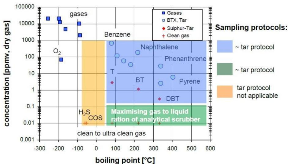
Figure 25. Boundaries of the tar protocol application for the detection of sulphur compounds [69].
