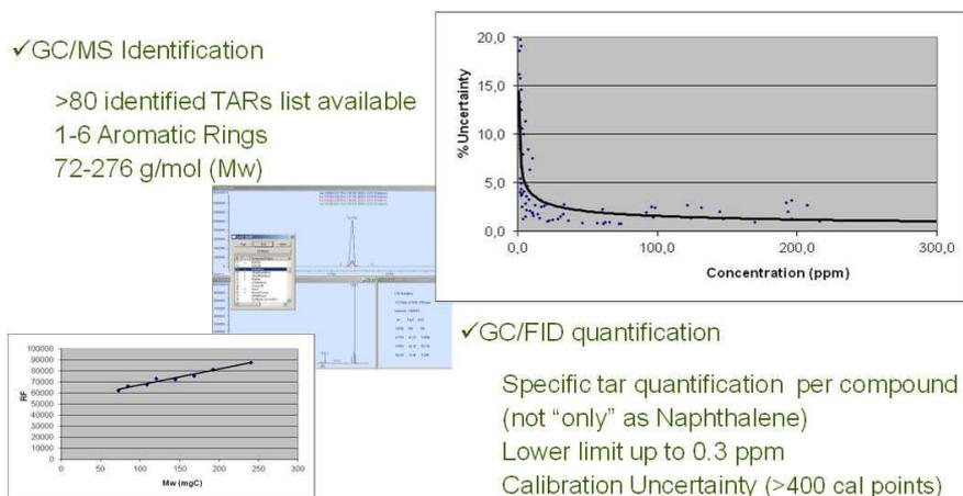
Figure 86. GC-MS and GC-FID applied at CENER: calibration procedure developed by CENER for quantification of tars.
