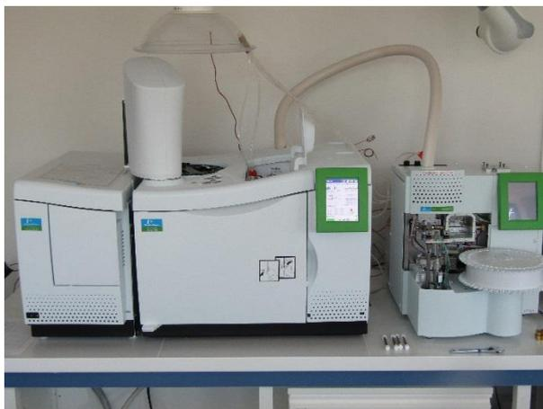
Figure 59. Thermal desorption unit coupled with GC-FID/MS. Picture courtesy of ENGIE Lab CRIGEN.
