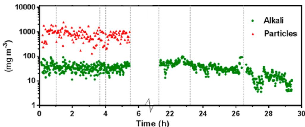
Figure 34. Mass concentration of alkali metals and particles measured at the GoBiGas plant using the online measurement method developed by Gothenburg University [126].
