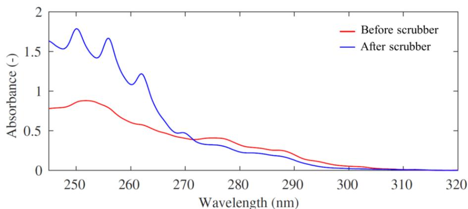
Figure 108. Spectra obtained at PSI before and after an oil scrubber applying liquid quench sampling coupled to UV-Vis spectroscopy [63].
