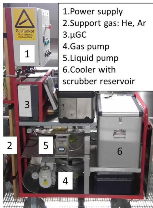
Figure 56. Portable micro-GC unit used at the GoBiGas plant [60].
