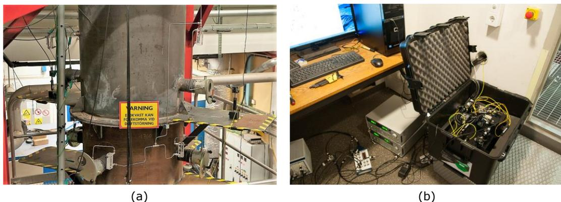
Figure 92. TDLAS system developed at Umeå University: (a) view of gasifier (100  $\text{kW}_{\text{th}}$  at Piteå) with TDLAS implemented; (b) portable, fibre-coupled optical setup in control room. Pictures courtesy of Umeå University.
