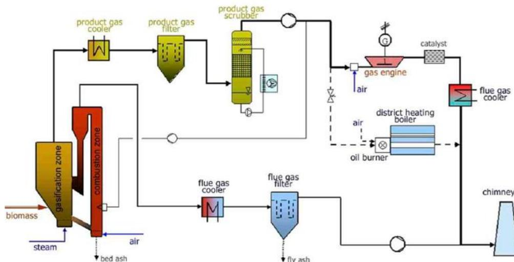
Figure 61. Schematic layout of Güssing CHP plant [110].
