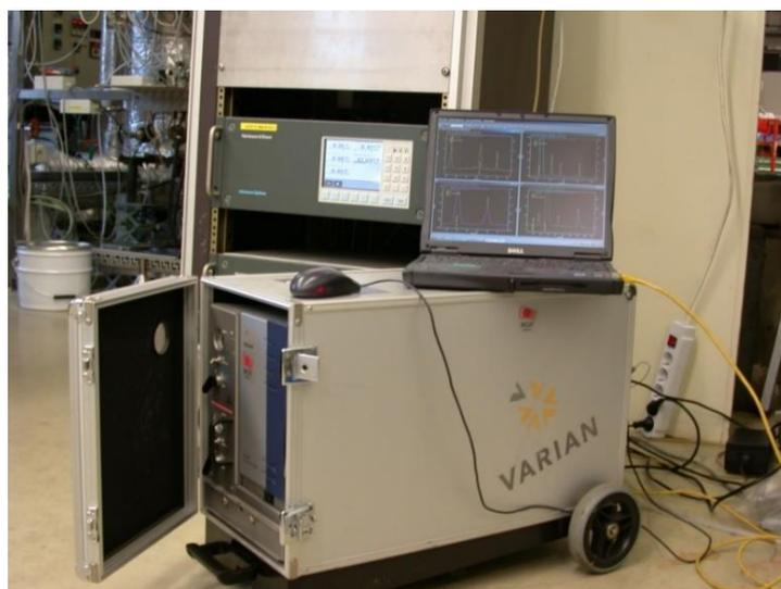
Figure 3. Micro-GC analyser used at ECN part of TNO [9].
