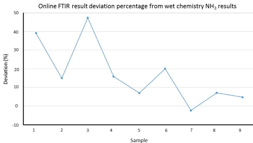
Figure 28. Comparison of results of online measurement of ammonia using FTIR and offline analysis using wet chemical analysis [19].
