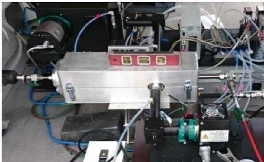
Figure 20. Gas cell for far UV absorption measurements up to 300°C at DTU [65].
