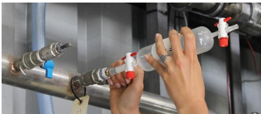
Figure 5. Gas sampling with gas pipettes for permanent gases + GC-TCD (offline) analysis at DTU [11].
