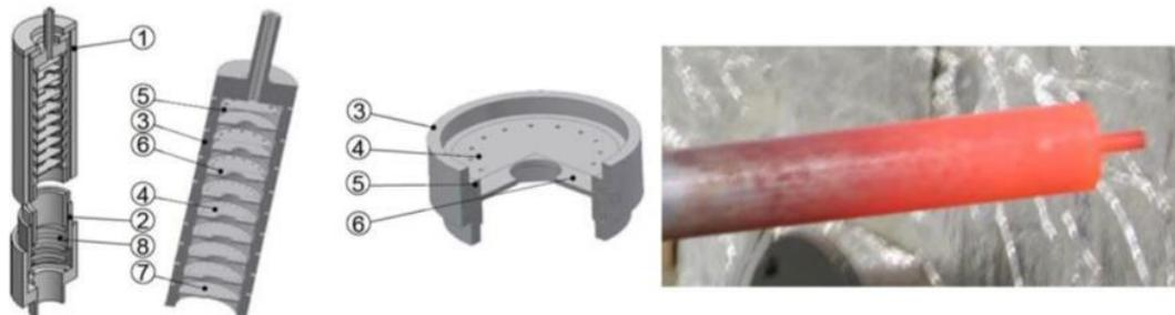
Figure 42. Schematic of high-temperature cascade impactor (left); high-temperature cascade impactor from BE2020+ after operation (right) [69]. Legend: 1. Outer casing; 2. Inner casing; 3. Shell; 4. Orifice plate; 5. Spacer ring; 6. Stagnation plate; 7. Critical orifice; 8. Spring.
