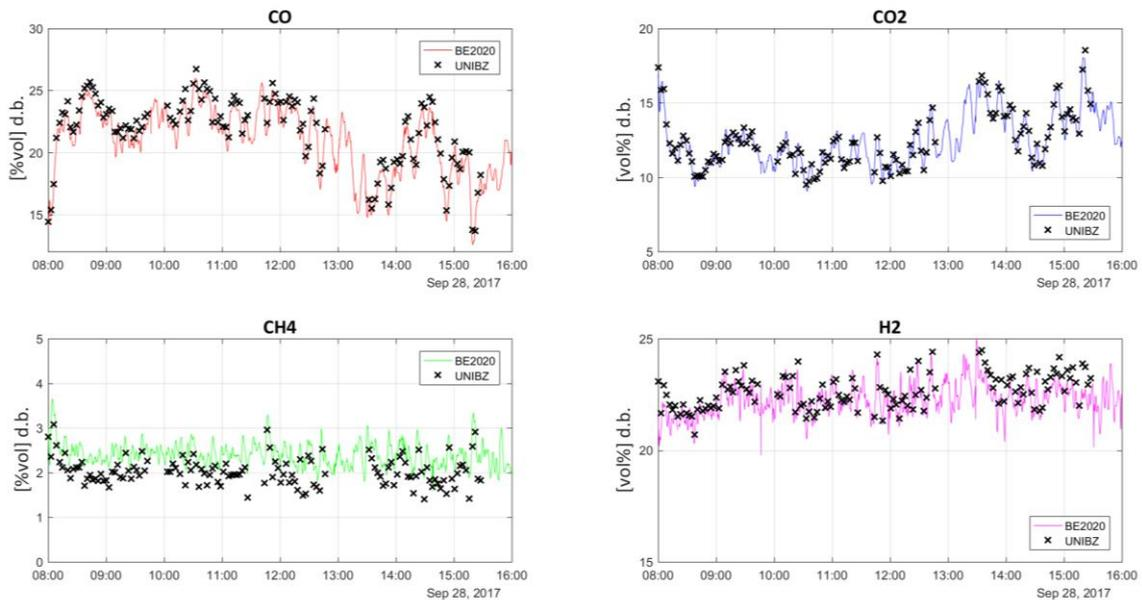
Figure 98. Results from a round robin measurement campaign of UNIBZ (micro-GC/FID) and Bioenergy 2020+ (NDIR, TCD, and FTIR) for comparison of measurement techniques [205].
