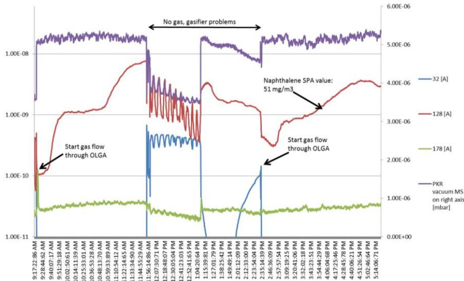
Figure 70. MS signals for online tar analysis during measurement campaign at commercial MILENA-OLGA plant operating with RDF [163]. Legend:  $m/z=32$  – oxygen;  $m/z=128$  – naphthalene;  $m/z=178$  – phenanthrene/anthracene; PKR: MS pressure (in mbar, right axis).
