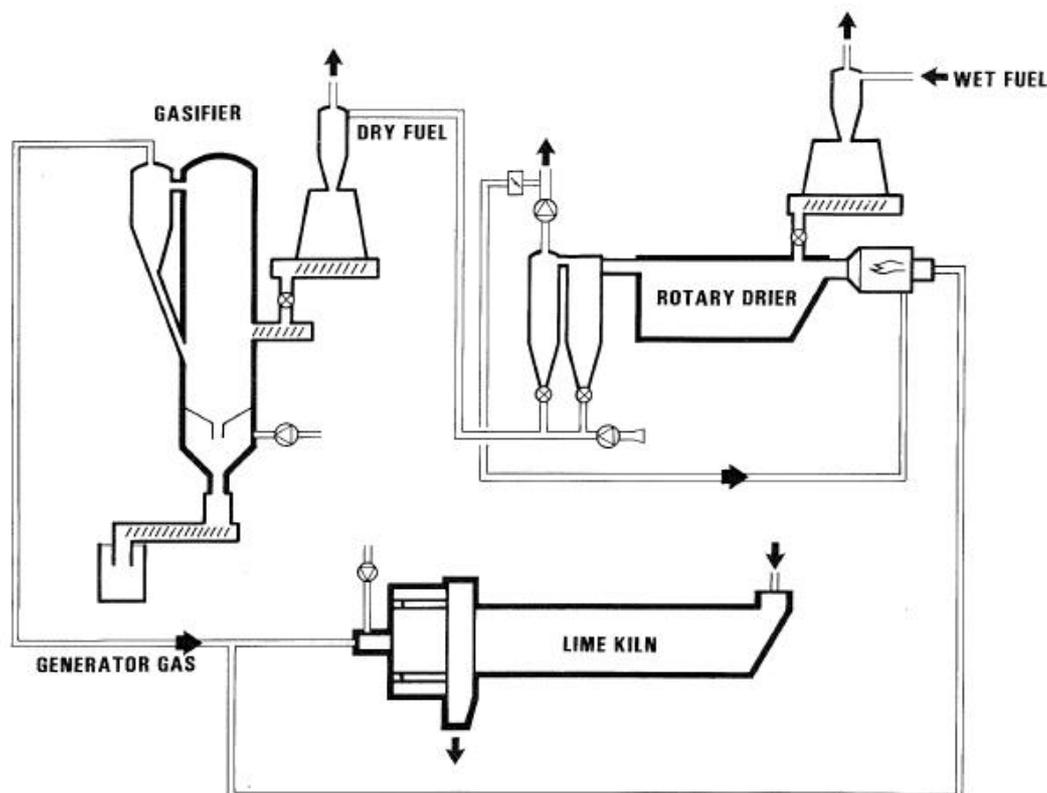
Figure 7 Biomass gasification plant at Värö Mill
