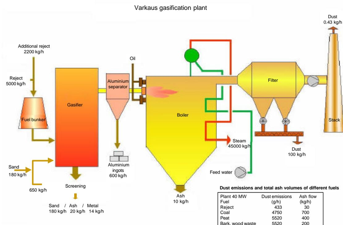
In Corenso's new gasification plant, the fibre material in multi-layer packages is recycled in coreboard, the aluminium being recycled as raw material for foil. The remaining plastic is gasified to create energy. The metal and packaging bands in the loads of collected raw material are sent to the metal industry for recycling. Thus, everything is recovered.
