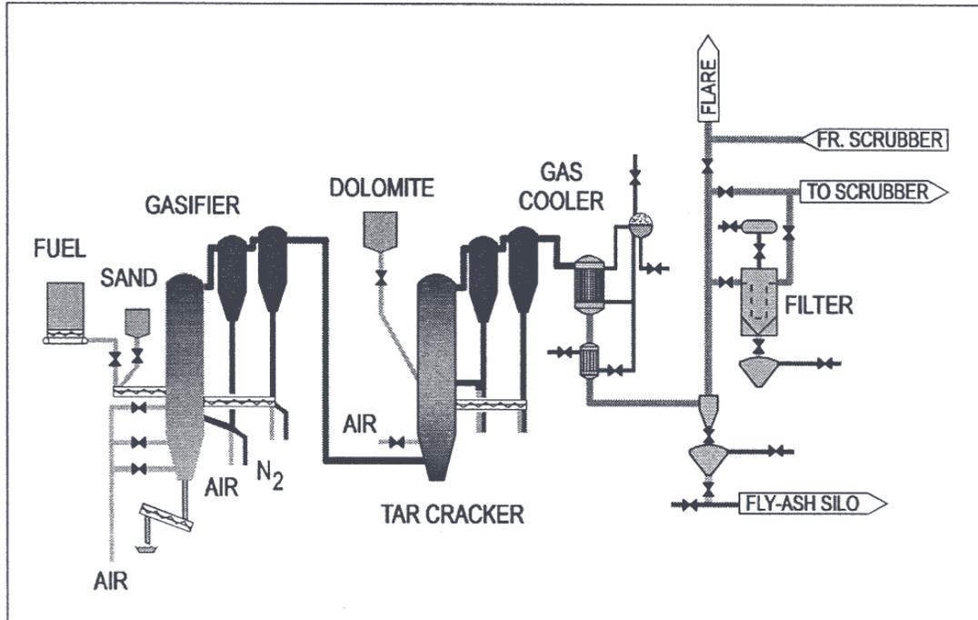
**Figure 1. Termiska Processor (TPS) CFB Gasification Pilot Plant**
