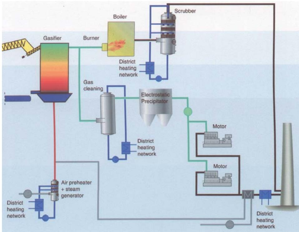
Today, the cleaned gas quality and also the problems connected with effluent waste-water have been verified and 2 gas-engines – each 768 kW<sub>E</sub> power (down-rated 1000 kW<sub>E</sub> natural gas engines from Austrian manufacturer Jenbacher) – are now in more or less continuous operation.
