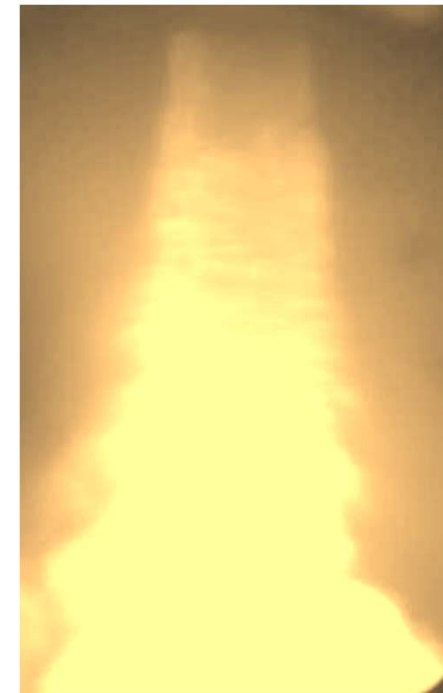
gasifier flame at 40 bar
