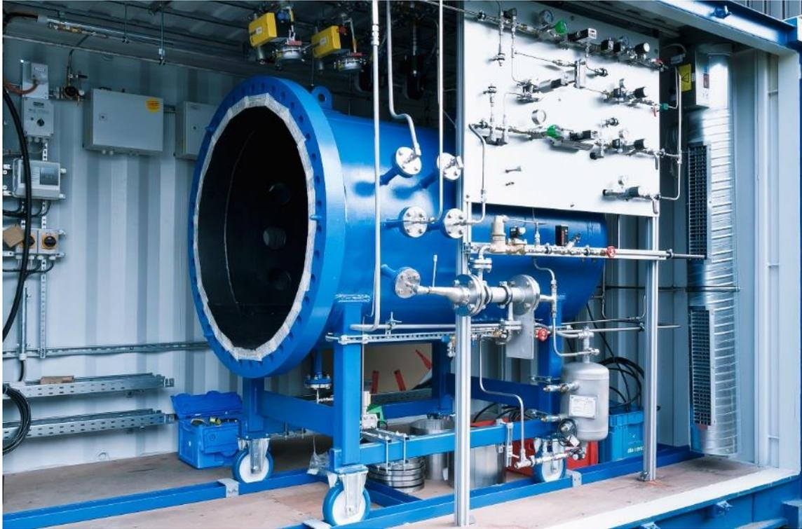
**Figure 4-2: SOEC pressure vessel inside container**
