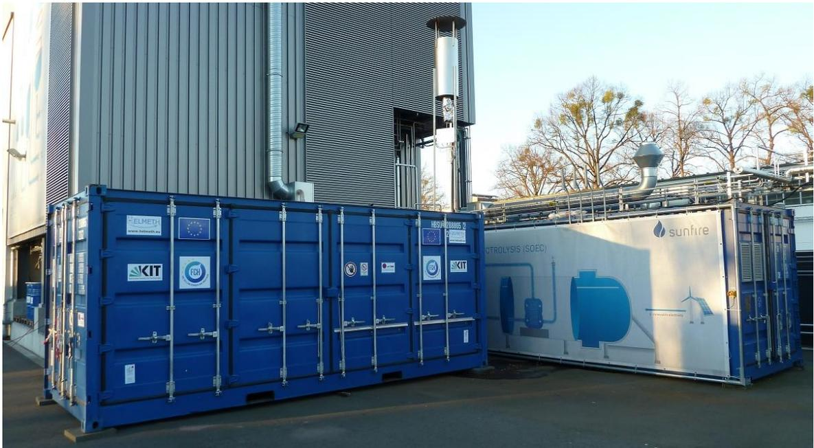
**Figure 6-1: Coupled PtG plant (left container: methanation; right container: electrolyser)**
