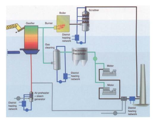
Today, the cleaned gas quality and also the problems connected with effluent waste-water have been verified and 2 gas-engines – each 768  $kW_E$  power (down-rated 1000  $kW_E$  natural gas engines from Austrian manufacturer Jenbacher) – are now in more or less continuous operation.
