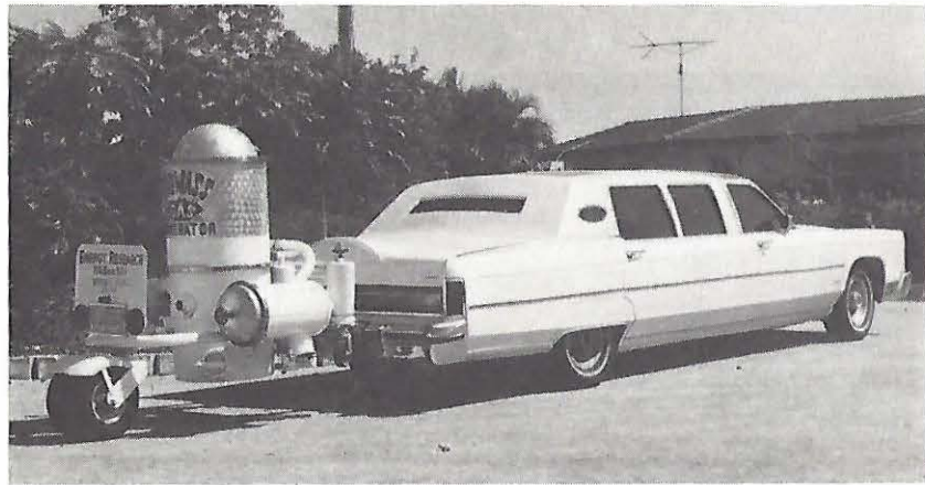
Miami, Florida, 1981. A charge of 110 lb of wood in the generator of this wood-powered 8,000-lb Lincoln Continental limousine takes it 85 miles or so on flat Florida terrain. In 1981, under a contract from the Department of Energy, its owner toured many southern universities demonstrating producer gas technology, especially to engineering students. (H. La Fontaine, 1995 Keystone Boulevard, Miami, Florida 33181, USA)
