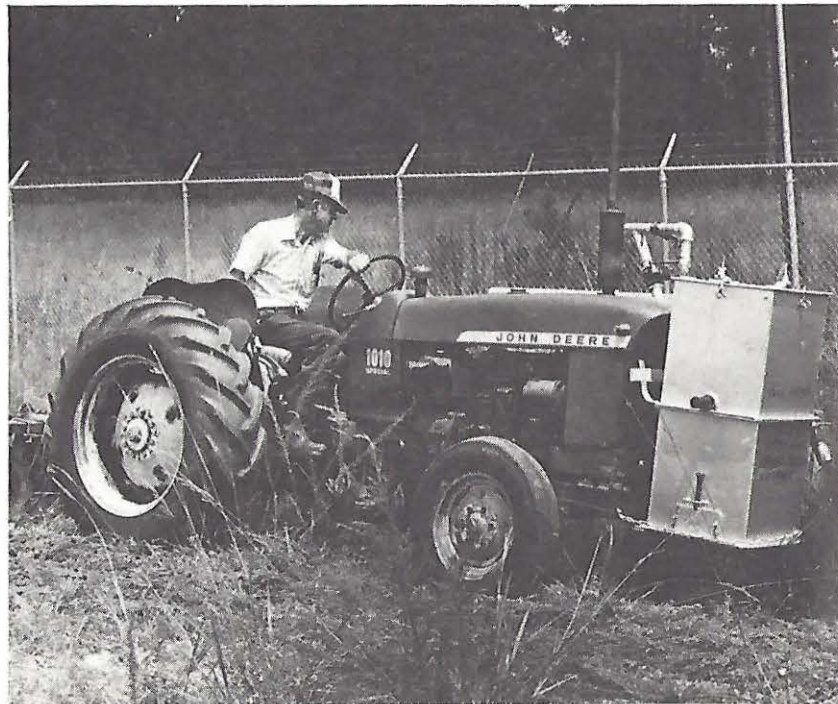
La Crosse, Florida, 1981. Wood-burning farm tractor used for plowing, mowing, and other farm chores. (R. Hargrave, photo courtesy Florida Times-Union /D. Stansel)
