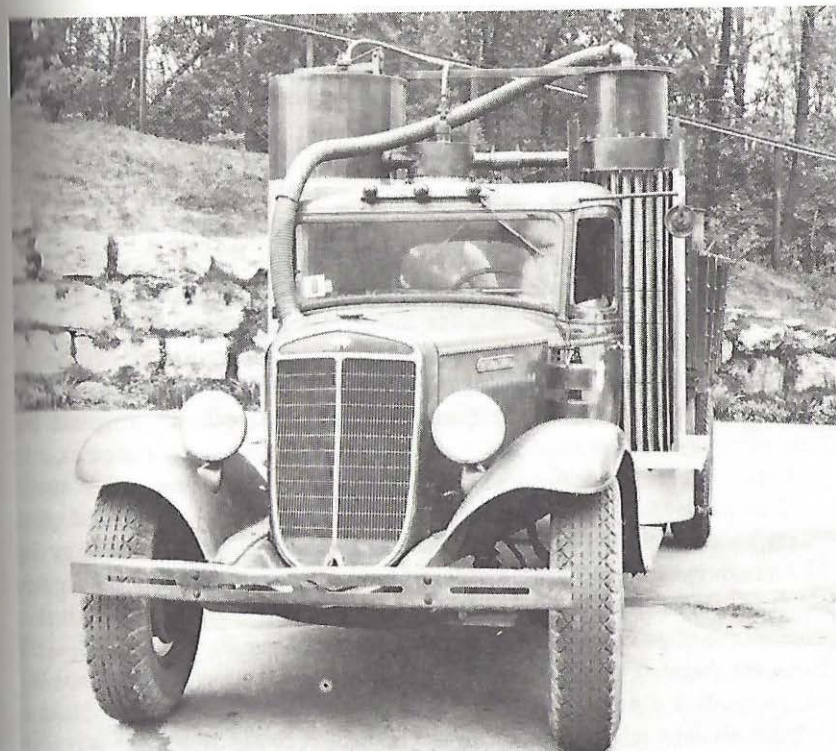
Madison, Wisconsin, USA, 1943. Truck fueled by sawdust. (Forest Products Laboratory, US Forest Service)
