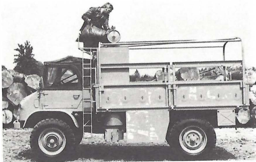
Brussels, 1979. This Mercedes Unimog recently did 100 km in 1 hour, running at full power. It used 20 kg of charcoal, with a gas producer unit weighing 450 kg, with a range of 3 hours at 60 kph. (Lambiotte, S. A., Brussels)
