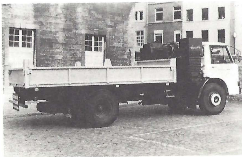
Andenne, 1981. "Dual fuel" diesel truck with gasifier fueled with wood, charcoal, peat, densified wood waste, or coconut waste. (S. A. Willy)
