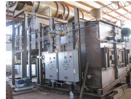
Digestate (cow manure) gasifier
