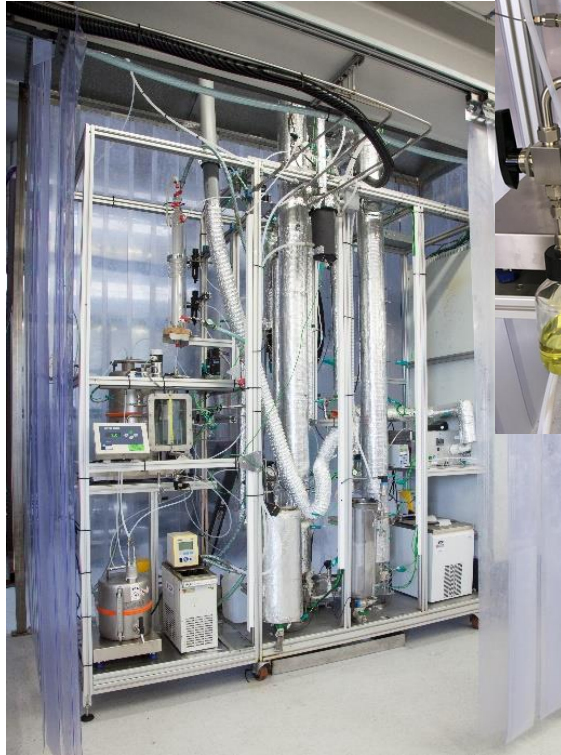
Bio-BTX scrubber unit + automated product separation (1 Nm 3 /h feed)
