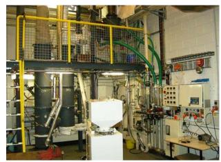
Fig. 7. 100 kW biomass gasifier in CAPE of UoC
