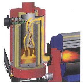
Fig.10. Working principle of the Waiariki gasifier
