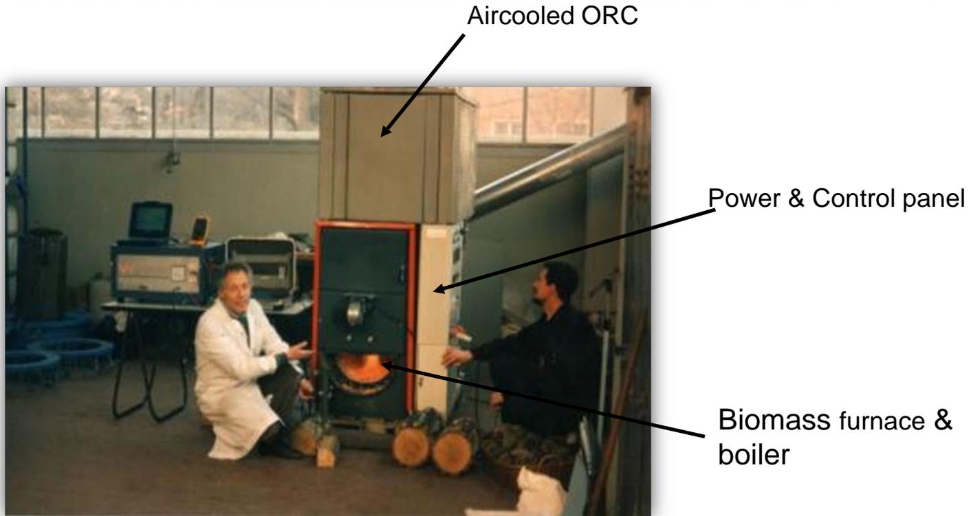
**1987:** A 3 kW<sub>el</sub> CHP biomass ORC turbogenerator prototype in Milan
