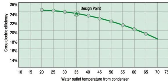
Gross performance of the Turboden HRS modules at various condensation water temperatures
