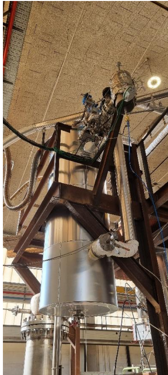
vessel for candle filters 3-way valve Nitrogen tank
