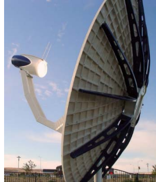
Parabolic Dish (C ≈ 2500, T ≈ 800 °C)
