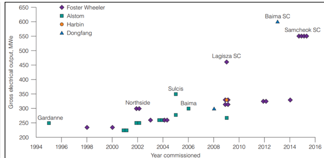
The scale-up of CFB boiler capacity in the last twenty years, with significant plants labelled (Source: IEA, 2013 "Techno-economic analysis of PC versus CFB combustion technology")
