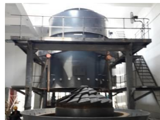
Steam boiler, 27 tons/day
