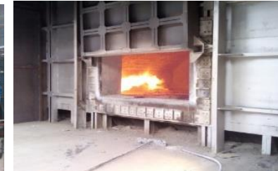
Aluminum melting furnace, 135 tons/day
