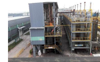
Aluminum melting furnace, Stainless steel furnace, 270 tons/day
