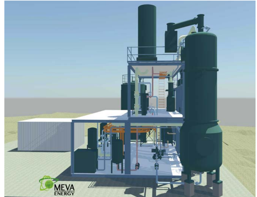
Modular build concept, pre-assembled before sent to site.
