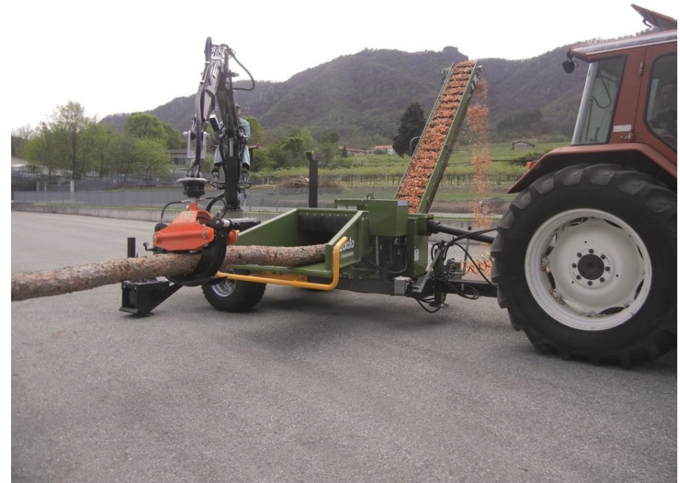
Pezzolato PTH 250 chipper for the Prato plant
