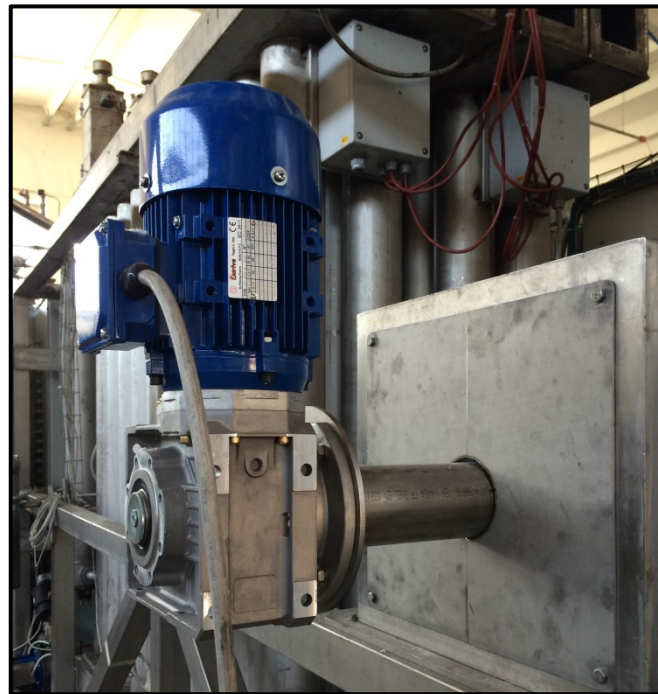
mechanical anti-fouling in any hot gas pipe
