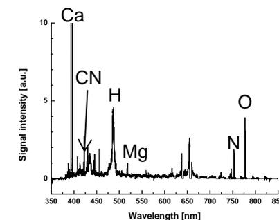
LIBS spectrum from gas phase measurement in REGA gasifier
