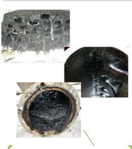
Fouling and plugging caused by biomass tars: heat exchanger, gas engine, pipes. Besides its main components (CO,  $H_2$ ,  $CH_4$ ,  $CO_2$ ,  $H_2O...$ ), product gas contains undesirable compounds which can cause operational problems in downstream equipment. The main contaminants of product gas are:
