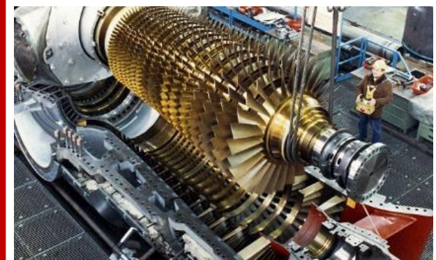
SGT6-2000E (up to 116 MW) Reliable, robust, fuel flexible
