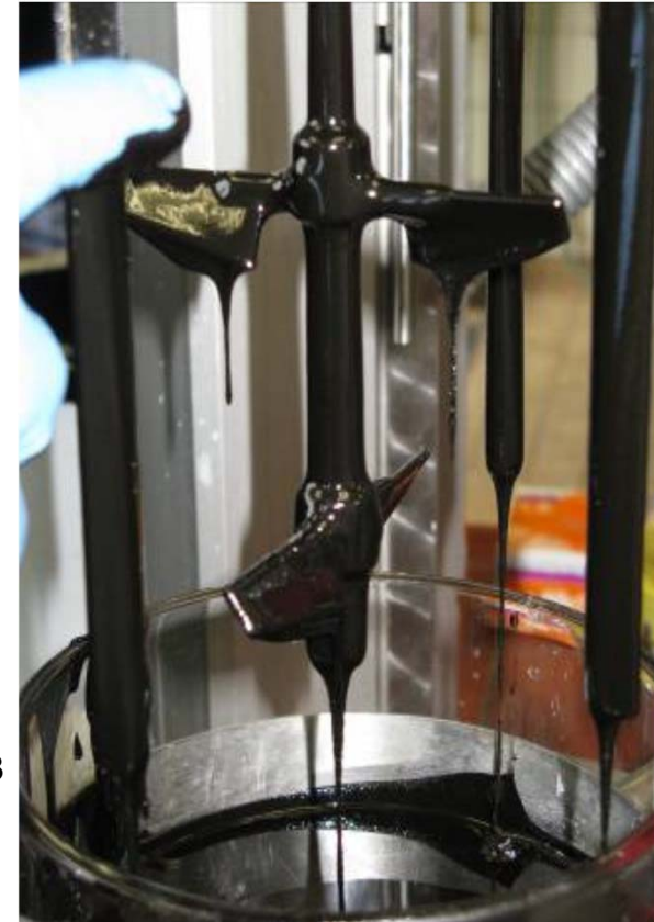
Organic condensate 30% solids
