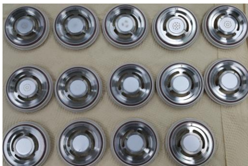
Solid sampling (6nm-10 \mu m) (FPS-4000+ELDI, Dekati)
