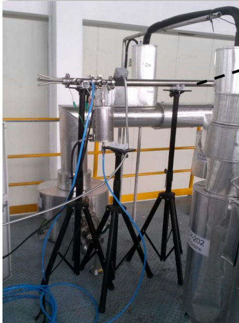
Solid sampling (6nm-10 \mu m) (FPS-4000+ELDI, Dekati)
