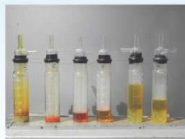
Figure 4 Serie of impingers bottles containing isopropanol (IPA) and the tar absorbed
