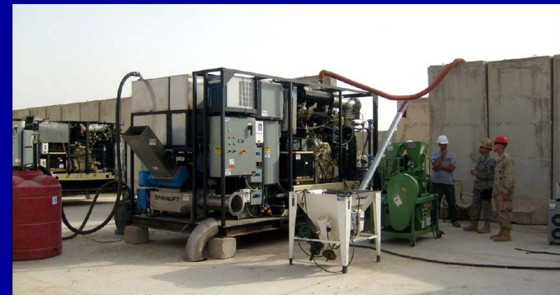
Prototype Tactical Biorefinery Mobile encampment feeding waste to energy (gaseous fuels and ethanol) US Army/Baghdad Contractors: Community Power Corporation, Purdue University, Defense Life Sciences May 2008
