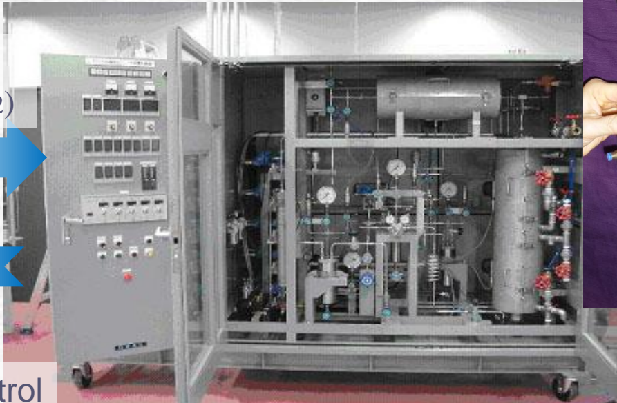
Lab-scale LPG synthesis reactor (Japan Synthesis Gas/University of Kitakyushu)
