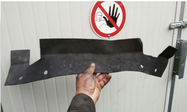
Broken backstays due to bad concrete
