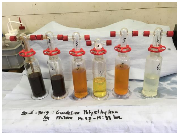
After Milena gasifier
