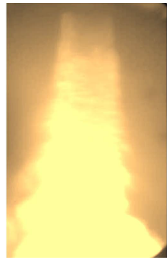
gasifier flame at 40 bar
