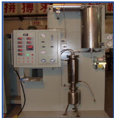
Fixed bed gasifier (600-800 °C)
