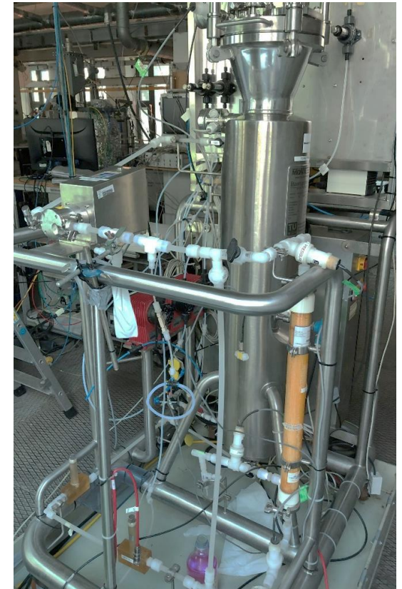
20 liter bubble column gas fermentation reactor at TU Wien
